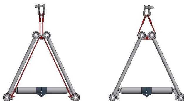
Figure 8: Slinging methods for triangular folding trusses.
