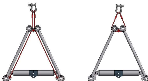
Figure 8: Slinging methods for triangular folding trusses.
